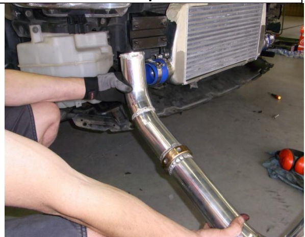
40. Install hdi intercooler cold pipe thru the back of the head light step3
