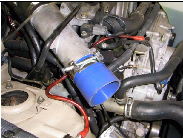
39. Install hdi intercooler cold pipe1 step 2
