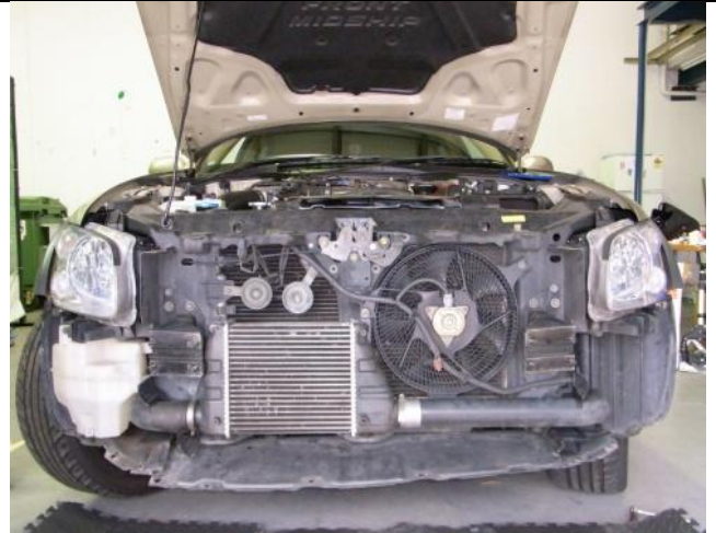
9. Remove std intercooler rubber hose
