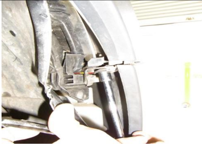
7. Remove front reinforcement bar holding screw
