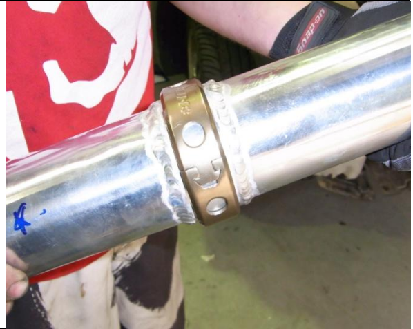
38. Install hdi intercooler cold pipe turn the pipe to the angle as shown step 1
