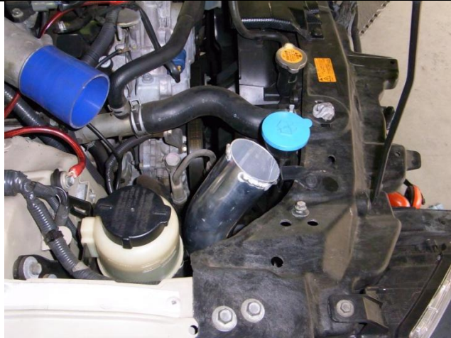
43. Install hdi intercooler cold pipe
