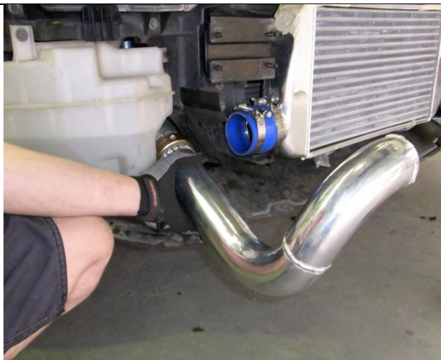
39. Install hdi intercooler cold pipe1 step 2
