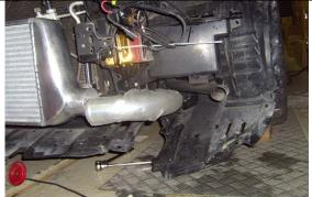
Install the passenger side intercooler pipe as shown using the supplied HDi Silicon Hoses and HDi Super Clamps.
