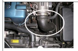
Connect the passenger side intercooler pipe to the Std. Rubber joiner.
