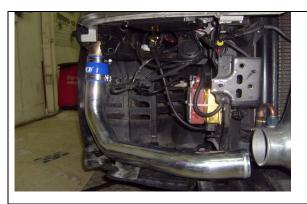
Install the driver side intercooler pipe as shown using the supplied HDi Silicon Hoses and HDi Super Clamps.
