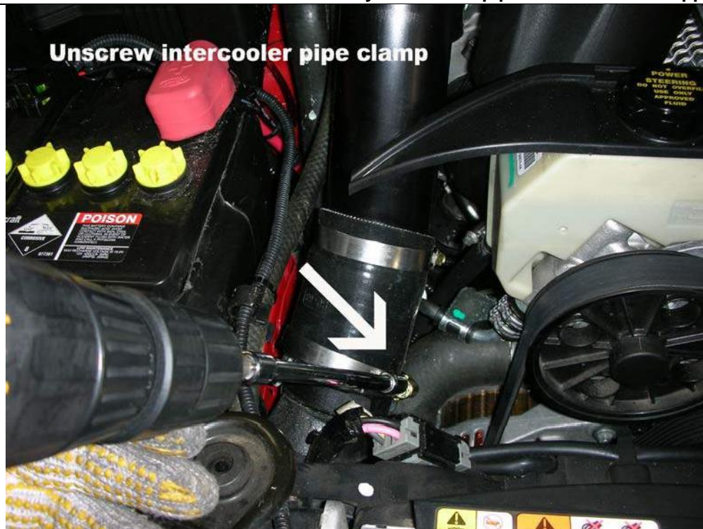
ENGINE BAY: Unbolt intercooler pipe from bracket
