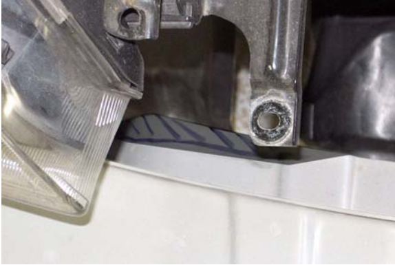
3. Trim both side top bumper bar support
